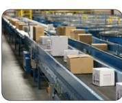
Conveyor systems are used in a variety of industries to move materials, reducing the need for human labor and boosting facility efficiency and productivity. By reducing the amount of human exertion needed to move materials, convevor systems also reduce injury risk. Conveyor systems have also been found to be safer than using forklifts to transport materials, which garners another safety benefit.
